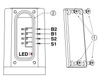
Note: remove the 4 screws (1) of driver's rear cover to access user settings and diagnostic led
