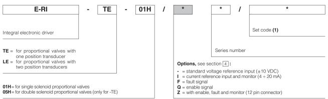
(1) set code identifies the corrispondance between the integral driver and the relevant valve; it is assigned by Atos when the driver is ordered as spare part
